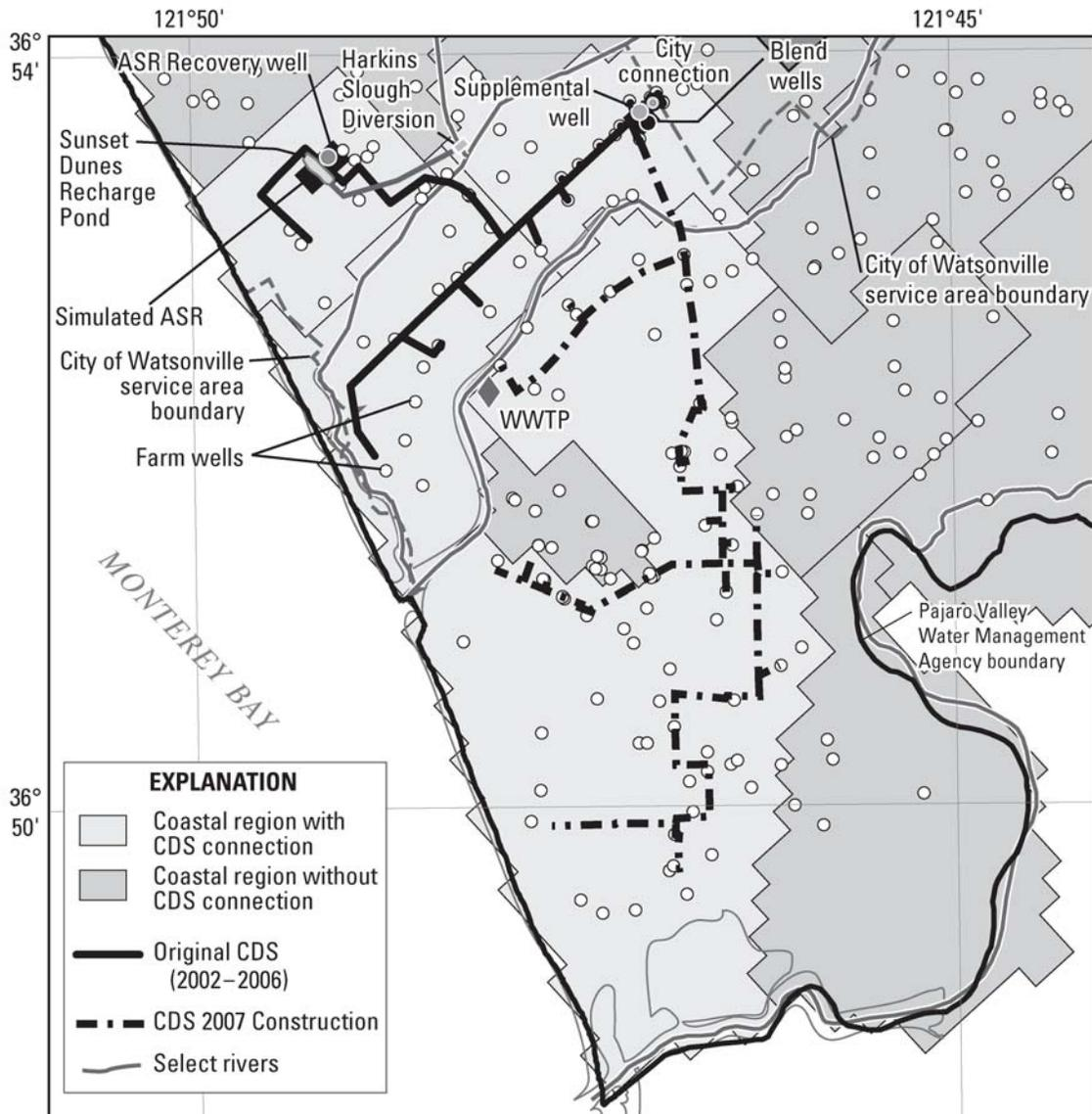
**Figure 2. Map showing CDS portion of PVMF2K onshore model region, selected water-balance subregions, selected wells, Aquifer-Storage-and-Recovery System (ASR), and Coastal Distribution System (CDS), Pajaro Valley, California.**
