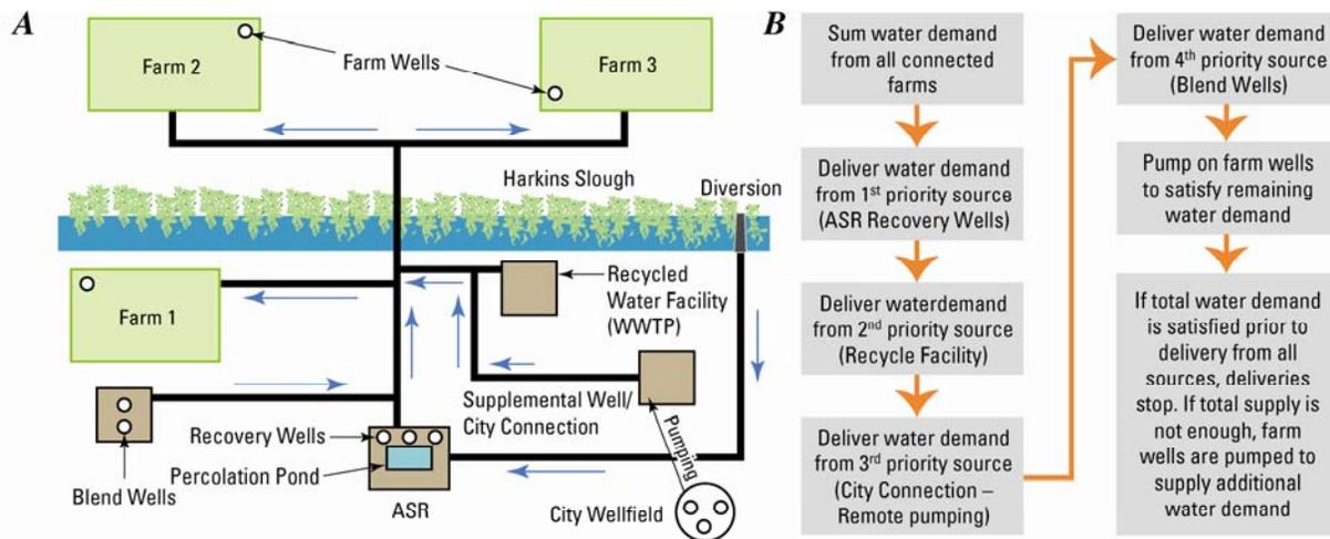
**Figure 3. Diagrams showing (A) the structure of local deliveries and (B) the order of operation of the simulation scheme for ASR and CDS deliveries to the regions serviced by the CDS, Pajaro Valley, California.**
